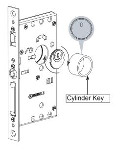
Note: Notches on cylinder must be parallel with the horizontal plane when fully screwed into lock body.
